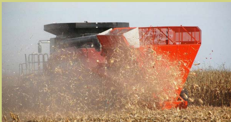
Cob Caddy™- Self contained sort and collection wagon pulled behind combine
