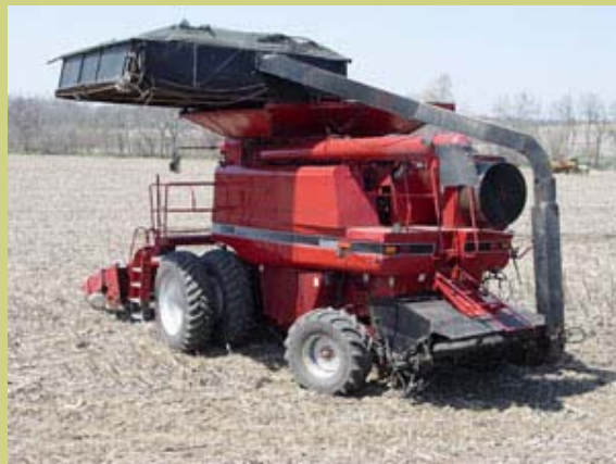
Ceres Residue System™- Attachment sorts stover at back of combine and collects cobs in hopper on top of combine
