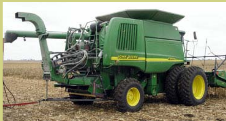
Iowa State University experimental cob collection attachment. Sorts cobs and blows them into wagon pulled behind
