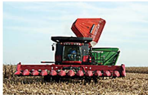
Figure 5. Full Cob Caddy™ wagon side-dumped cobs into tender wagon.
