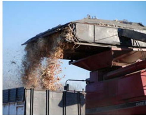
Figure 3. Ceres Residue System™- Full cob hopper emptied into truck
