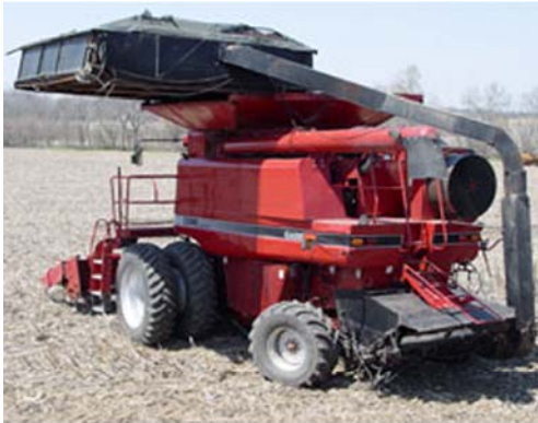
Figure 2 Ceres Residue System™- Attachment sorts stover at back of combine and collects cobs in hopper on top of combine
