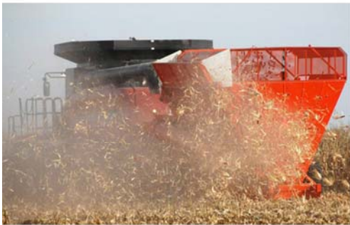
Figure 4. Cob Caddy™- Self contained cob collection trailer. Cobs collected in wagon basket and stalks, leaves and husks are spread onto field.
